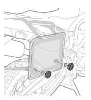
MARK THE UPPERS Once the lower mount locations are confirmed, use hardware to hold the frame sheet in place while marking locations for upper mounts.
