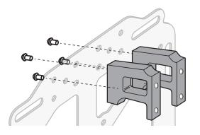
Use the LONGER black 15mm bolts included with your adapter to secure the locking clasp to the adapter.
